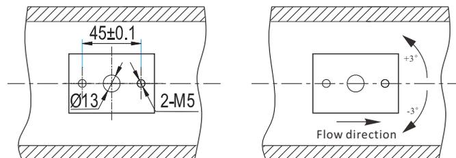
(3-4) Install the sensor, the flow measurement direction indicated on the sensor should align with the flow direction in the flow channel. Adjust the probe depth in the flow channel according to the measurement
