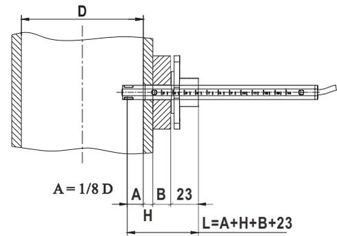
**Calculation of the probe depth, L**
