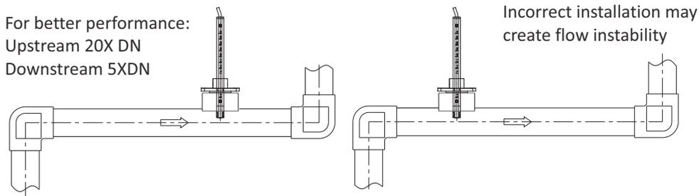
(3-3) Prepare the installation hole in the flow channel (13mm), and the installing base as below:
